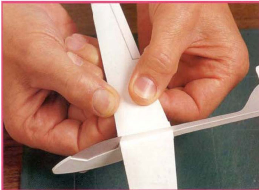
Figure 5 Adjusting Wing Curvature (Camber)
